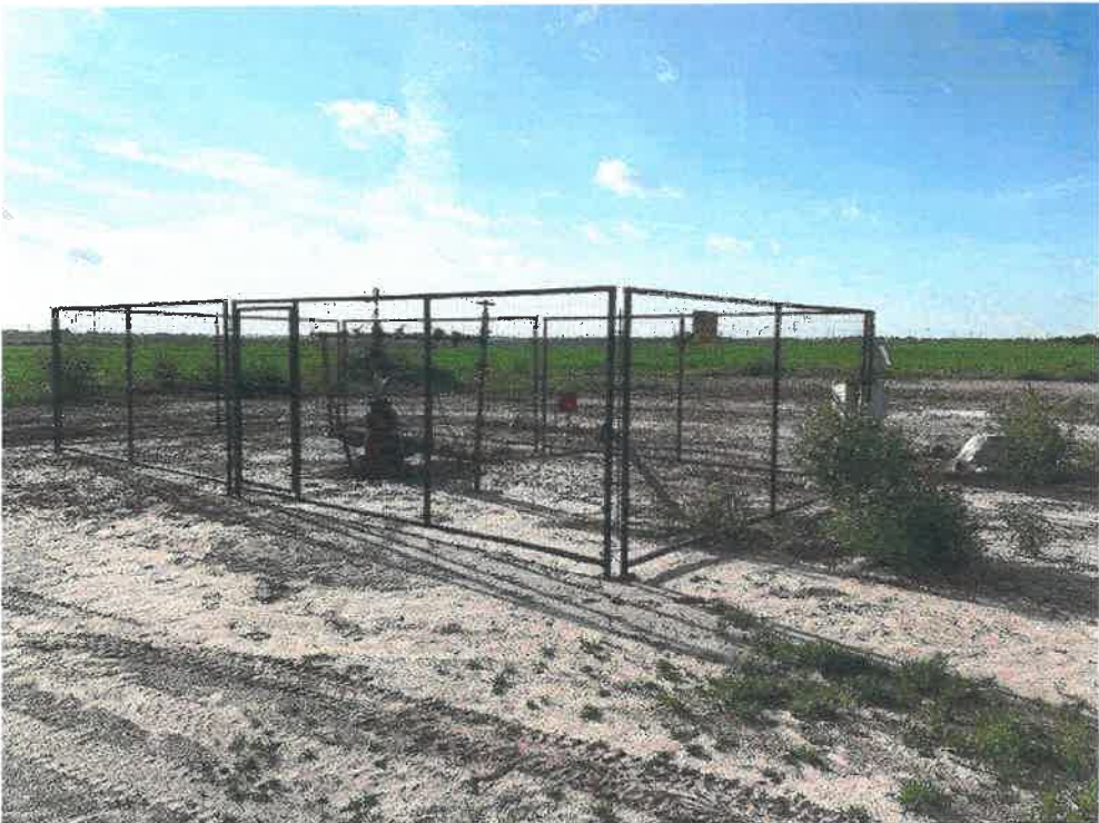
Photo 2. Typical fence panel currently at use at select SACROC well locations.
